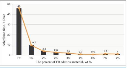
Fig. 4. Effect of flame-retardant additives on after-flame time of PP knitted fabric (Significant: 0.000)
