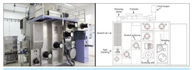
Fig. 1. Laboratory-type melt spinning machine used for yarn production [10]
